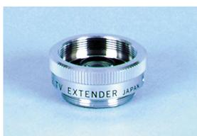
This is a subsidiary lens to be screwed in the rear of C-mount lenses so that the focal length is doubled for telephoto and close-up surveillance.
